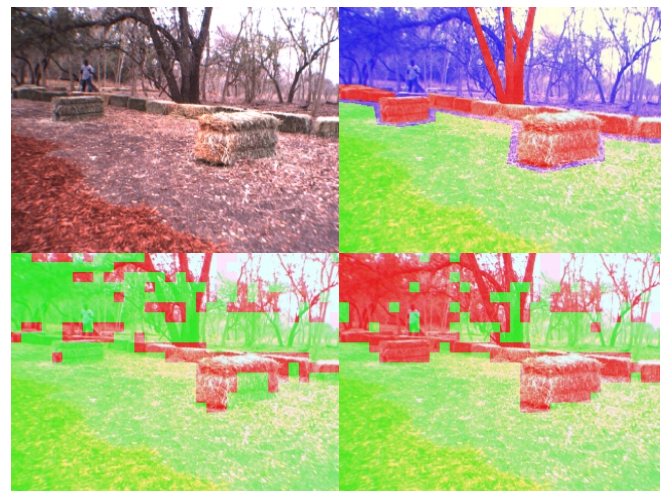
Figure 3. Input image (Top left), hand labeled ground truth (green: ground plane, red: obstacle, and blue: unknown) (top right), basic self-supervised SVM learning (bottom left), proposed confidence-based auto labeling approach (bottom right), DS4.
