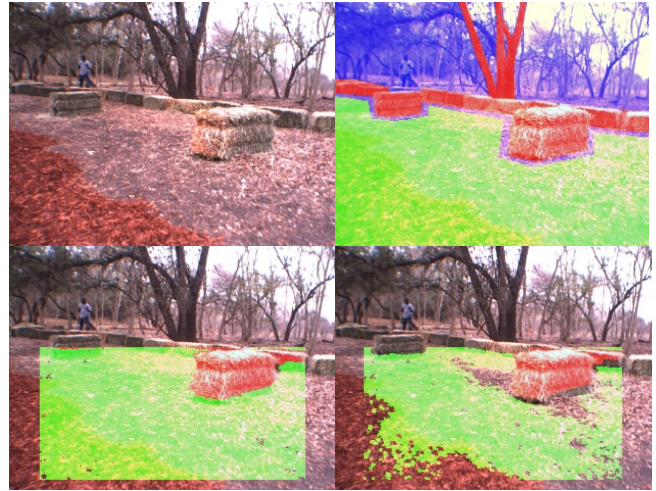
Figure 1. Input image (Top left), hand labeled ground truth (green: ground plane, red: obstacle, and blue: unknown) (top right), basic auto labeling output image (bottom left), proposed auto labeling algorithm output image (bottom right).
