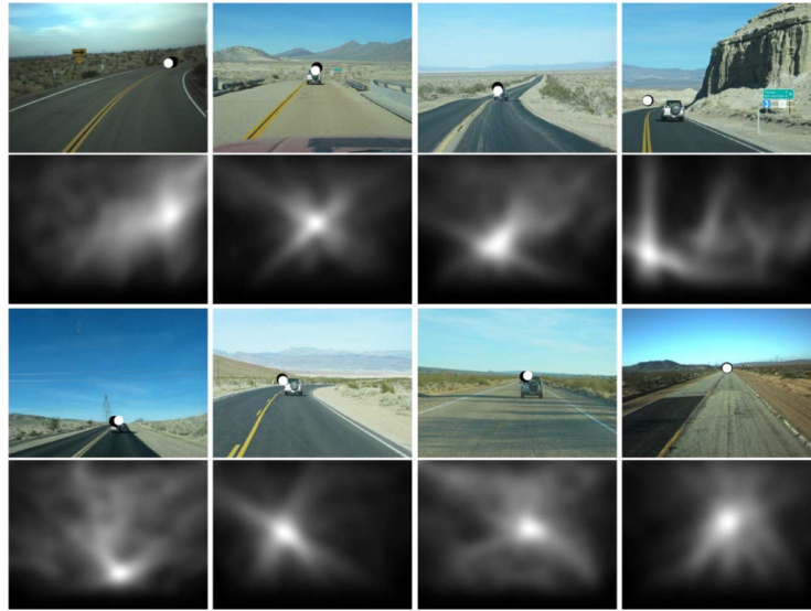
Fig. 5. Examples of vanishing-point detection for structured roads. First and third row: outputs of this paper's algorithm (black dot is the ground truth and white dot is the estimated vanishing-point location); second and fourth row: accumulator spaces.
